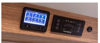
The **CP-Plus** and **LED control panel** allows central control of the on-board electrics and heating. In addition, you always have an eye on the water levels.
