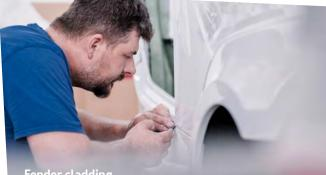
**Fender cladding.** The fastening is not visible from the outside, the seamless transitions guarantee robustness and durability.
