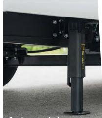
**Crank support in the rear.** Provides additional stability and less vibration when the vehicle is stationary.
