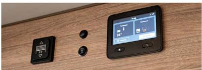
Central control panel and the new TRUMA iNet X system. One look is all it takes to check the water level, electronics supply and heating.
