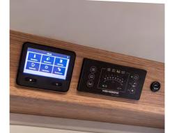
TRUMA iNet X and centrally arranged LED control panel. One glance is enough to check the water level and the electronics supply.
