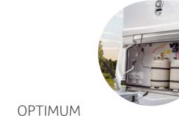
Thanks to the complex parallel lifting mechanism, you have a large access area. The gas pressure spring also ensures that the hood gently glides upwards. With the stable aluminium chequer plate floor, the gas box for 2 x 11 kg gas bottles becomes even more robust and offers a low loading edge. With our E.POWER vehicles, you will no longer have any need for a gas supply and will gain extra storage space in the front locker. For more information about our
