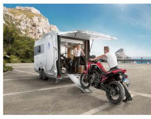
**DESEO 400 TR.** The 160 x 180 cm wide tailgate and the stable drive-on ramp which is secured during the journey by means of a rod & twist lock make loading particularly easy. Optionally you can also get a second loading ramp
