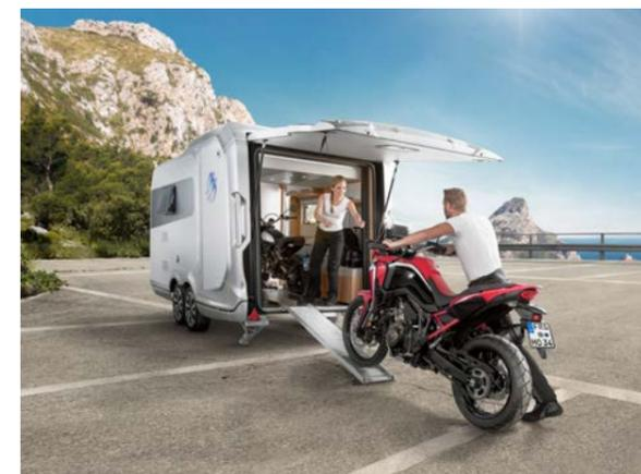
**DESEO 400 TR.** The 160 x 180 cm wide tailgate and the stable drive-on ramp which is secured during the journey by means of a rod & twist lock make loading particularly easy. Optionally you can also get a second loading ramp
