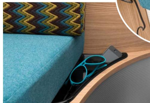
**SPORT&FUN 480 QL.** Easy charging. Right where you need it: 230 V socket and USB connection. Remote control and glasses can be stored in the integrated compartment.
