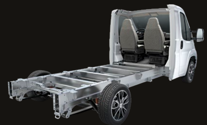
Lightweight high-frame chassis (CaraHome 650 DG).
