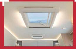
The large panoramic skylight with LED light lets both air and daylight into the vehicle (90 Years Package)
