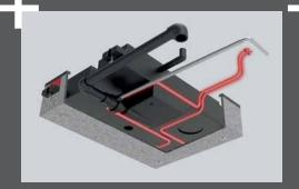
Heated and insulated 42-litre wastewater tank so that nothing freezes - even when the temperature falls below zero (option)
