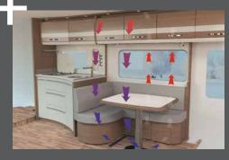
AirPlus – perfect air circulation in the interior with rear ventilation of the overhead lockers and sideboards
