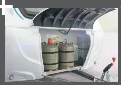
Gas bottle locker for 2 x 11 kg bottles with base made of rot-proof, sturdy aluminium chequer plate
