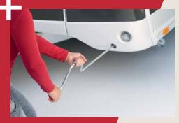
Crank insertion aid for convenient operation of the crank supports
