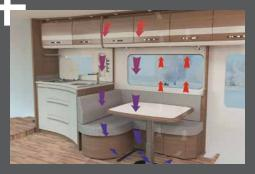
AirPlus – perfect air circulation in the interior with rear ventilation of the overhead lockers and sideboards
